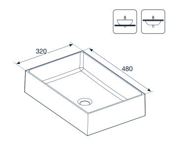
Dimensions in mm Tolerance ±5 mm
